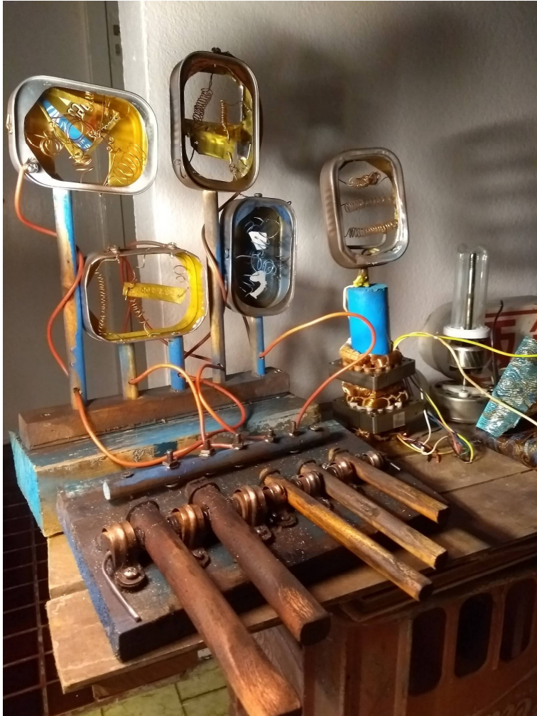
Figure 2. Speculative design: Prisoner of war Morse code radio transmitter using re-functioned sardine cans, broom handles, copper pipe fittings and recycled copper wire. (Author's collection)
